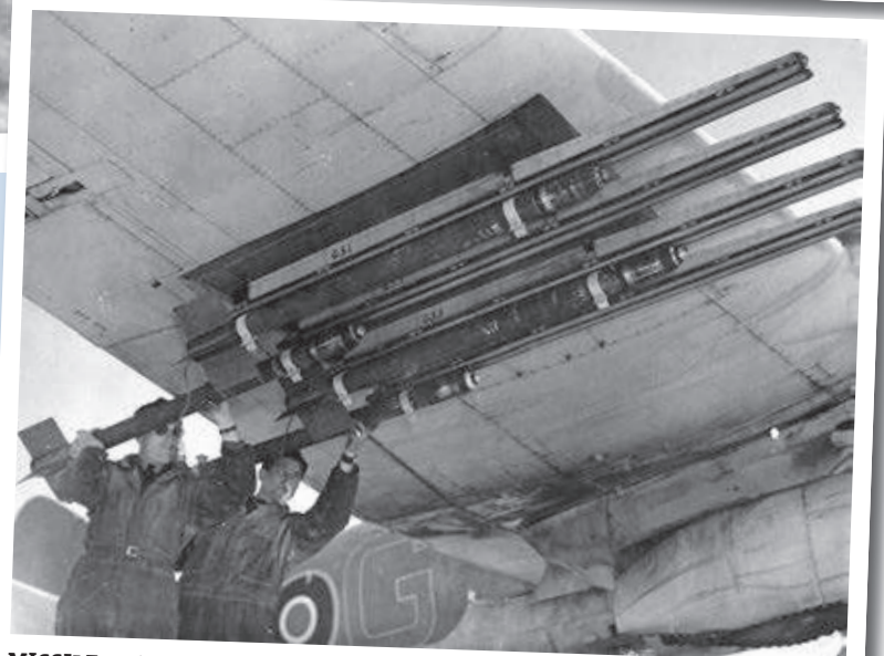
MISSILES: Three-inch Rocket Projectiles, effective anti-shipping weapons, are loaded onto a RAF Beaufighter ( Matthew Willis Collection )
